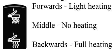
The heating can be activated when the motor is running only.
